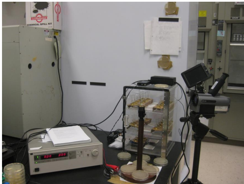
Figure 29. Nutrient agar plates used in ten places to try to capture spores during thermal inactivation testing
